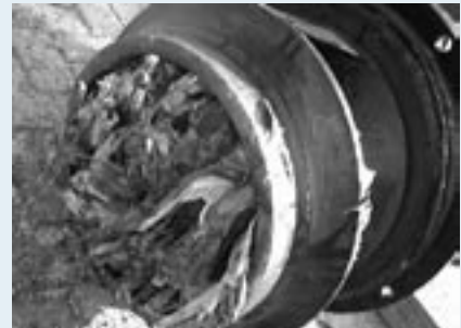
Illustration: Typical damage of clogged waste water pumps
