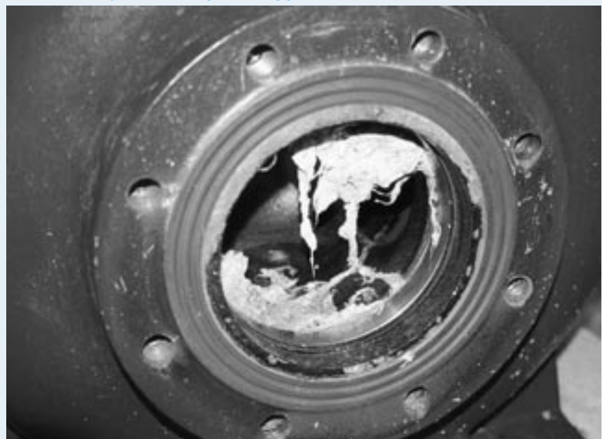
Illustration: Typical damage of clogged waste water pumps
