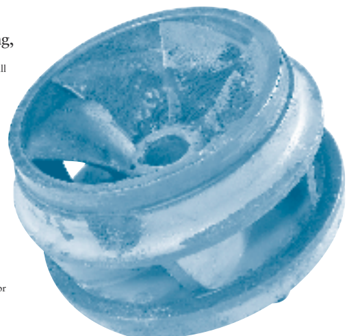
Photo: Etanorm impeller destroyed by cavitation
